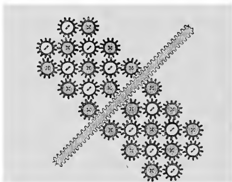
FIG. 39.—A provisional representation of a current surrounded by dielectric medium, either propelling or being propelled. Section through the wire.
