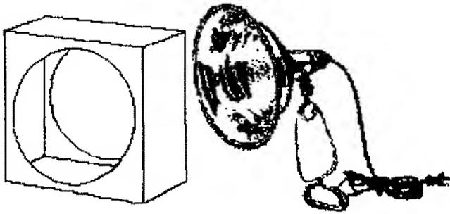
8. The box inside can be painted white or covered with kitchen aluminum foil to increase reflectivity, and minimize heat. If desired, the outside may be decorated with wall-paper, paint, vinyl shelf covering, etc.
