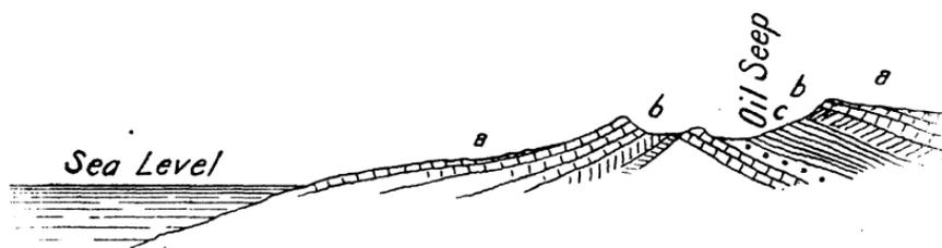
FIG. 12. Geologic section across strike of beds along Malbog Creek, Alegria, Cebu; a, coral-line limestone; b, volcanic tuff; c, Miocene shales and sandstones over limestone.
