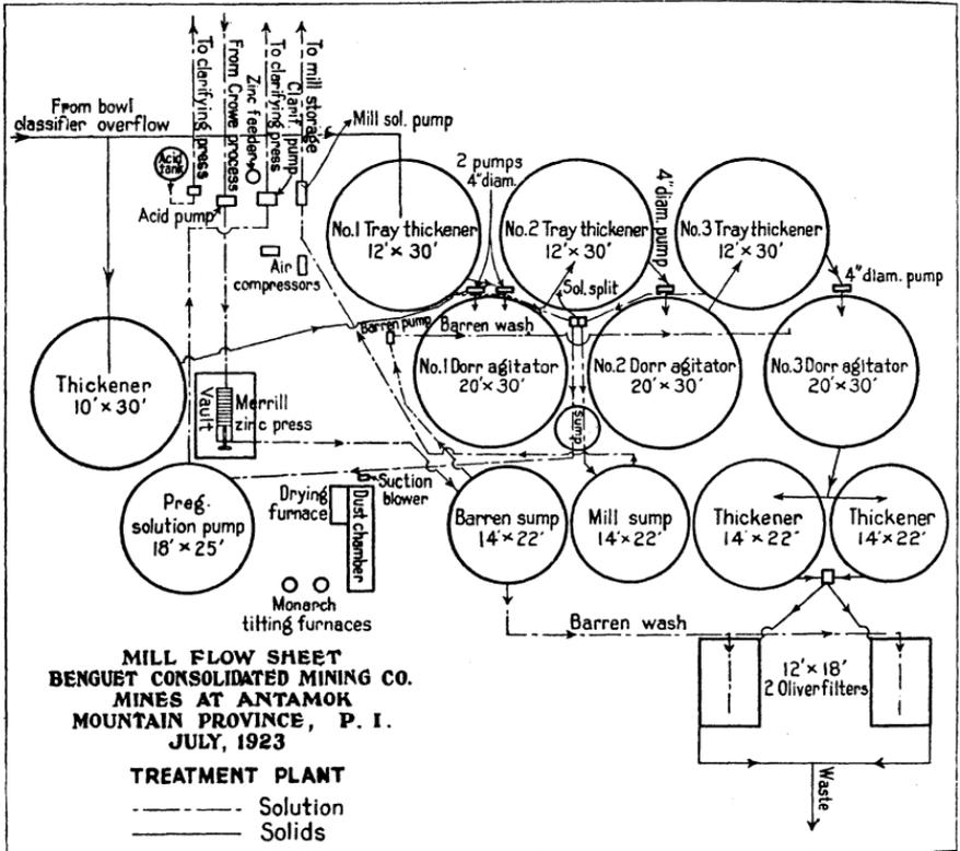
FIG. 22. Mill flow sheet of the Benguet Consolidated Mining Co.; treatment plant.
